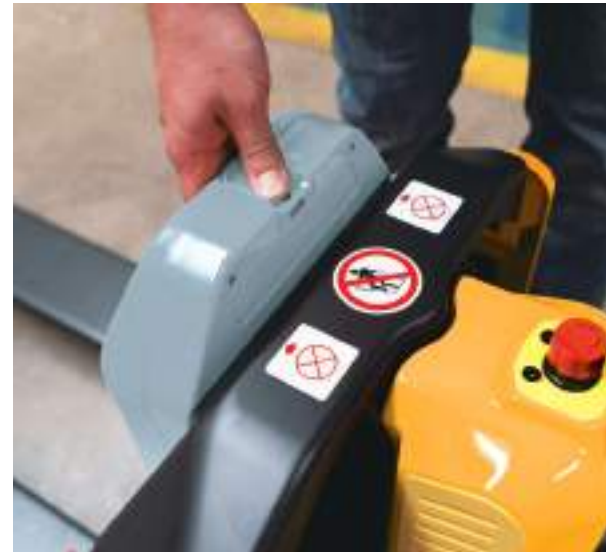
Socket on battery case for easy battery charging without necessity to take the battery out.
